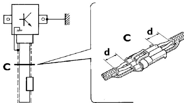
2. SCREENING THROUGH METALLIC BRAIDING OF A CABLE TO AN ELECTRONIC COMPONENT – C. CONNECTOR
